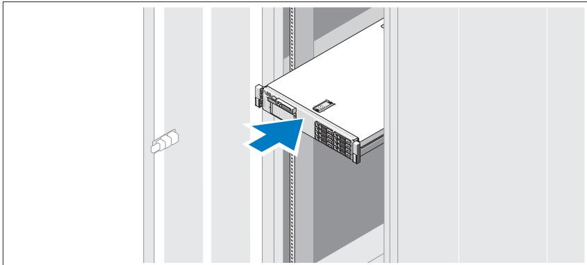
Assemble the rails and install the system in the rack following the safety instructions and the rack installation instructions provided with your system.
